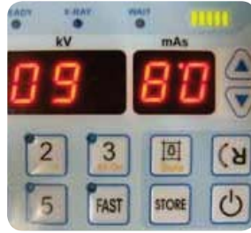
DISPLAY REVERSE SWITCH This switch makes easy reading of digits from opposite side.
